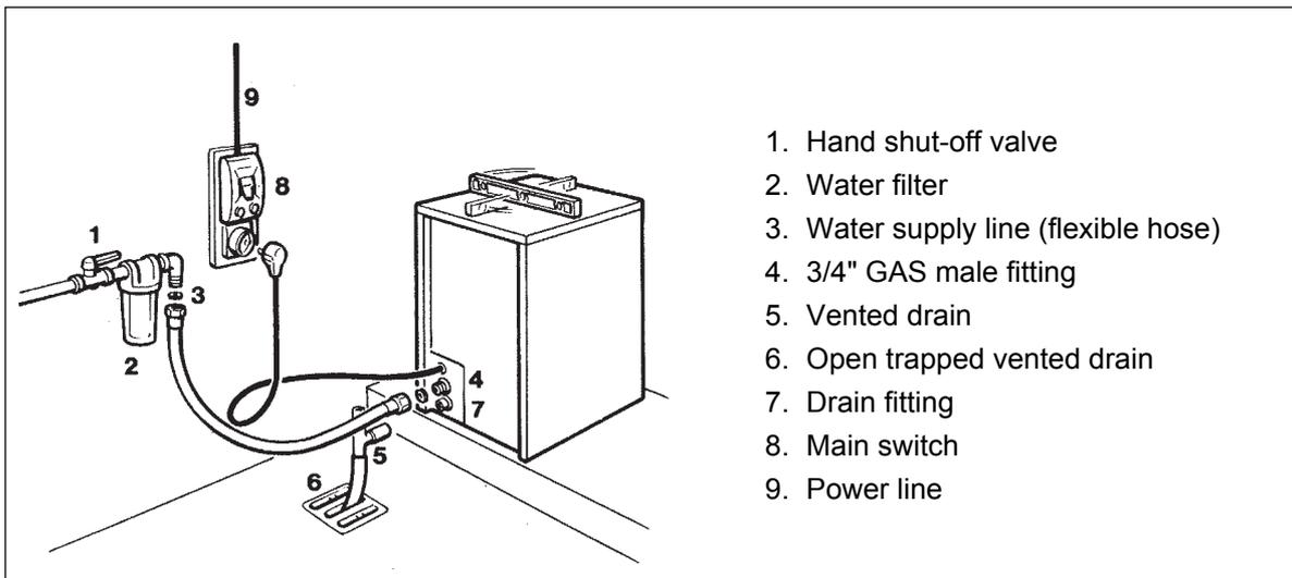
**WARNING.** This icemaker is not designed for outdoor installation and will not function in ambient temperatures below 10°C (50°F) or above 40°C (100°F). This icemaker will malfunction with water temperatures below 5 °C (40°F) or above 40 °C (100°F).
