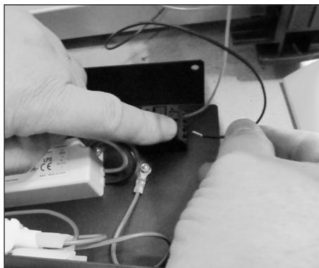
5. Remove the black and red wire from the connector by pressing down the clips.
