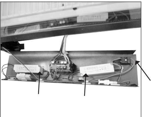
18. Click the wires to the door light onto the wire retainers and mount them in the connector.
