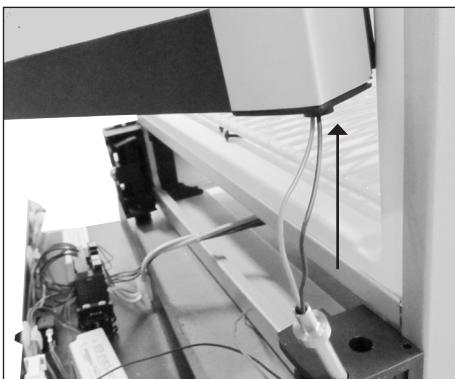
8. Lift up the door. The wires from the door are pulled up together with the door pin.
