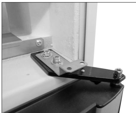
6. Unscrew the canopy bracket and the door hinge on the right side.
