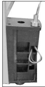
14. Push the wires from the door down into the door pin and drag them through the door support.
